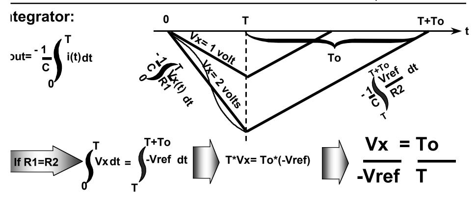
T is fixed at one cycle of 50 Hz or 60 Hz to eliminate line noise; Vref is fixed; R, C and Time are all ratioed, so accuracy is excellent.
